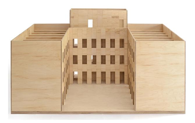
A wood model depicts a side view of a three-story, mixed-use building that will include structural wall panels made from cross-laminated timber. (Courtesy of Waechter Architecture)
